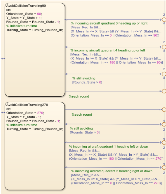
Figure 11: Collision Avoidance Modes
